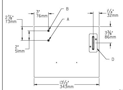
NOTE: It is important to insure proper ventilation. Allow a minimum clearance of 6 inches (152 mm) in front and 3 inches (76mm) in the rear of the unit. If unit is to be installed in an enclosure, allow the following clearances around unit - 1 inch (25mm) each side, 3 inches (76mm) in the rear, 3 inches (76mm) inches above wall.
